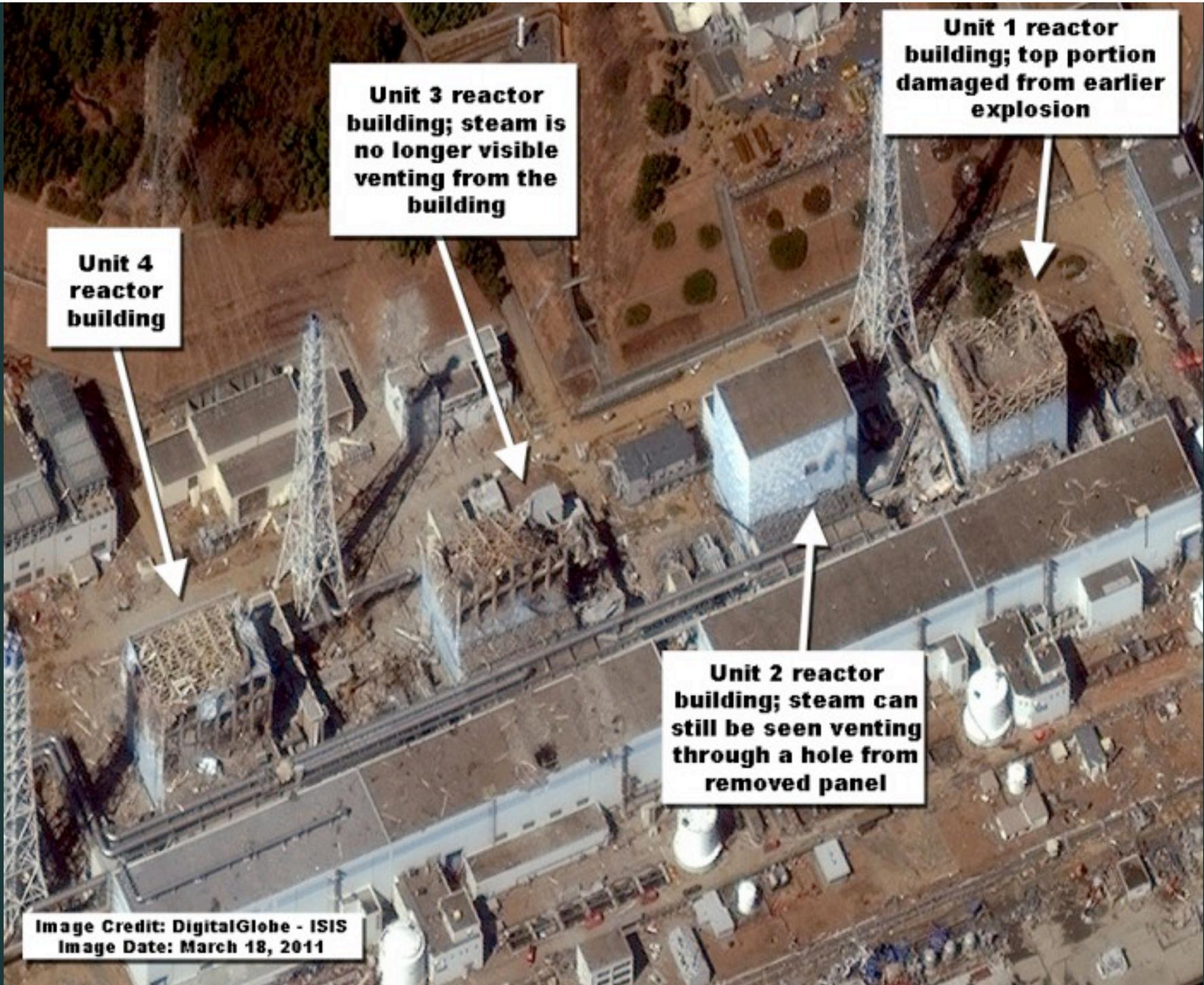
**Unit 1 reactor building; top portion damaged from earlier explosion**
