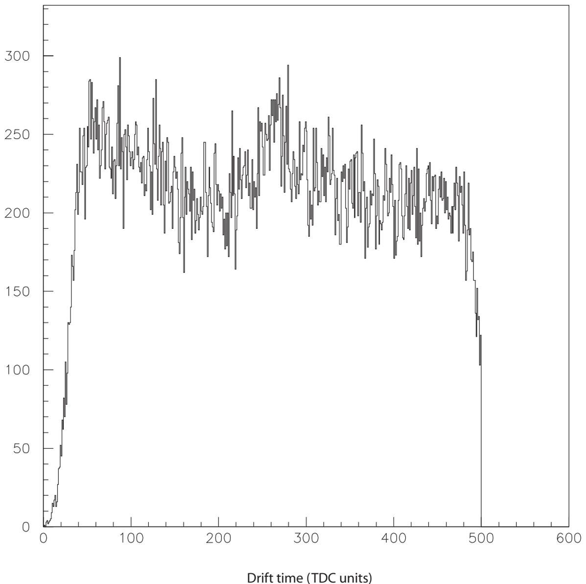
**Figure 1-** Drift time distribution for cosmic rays on a MB3 chamber at LNL with the minirate setup in default configuration. The distribution refers only to layer 1 of SL 1. No difference is observed on the other layers.
