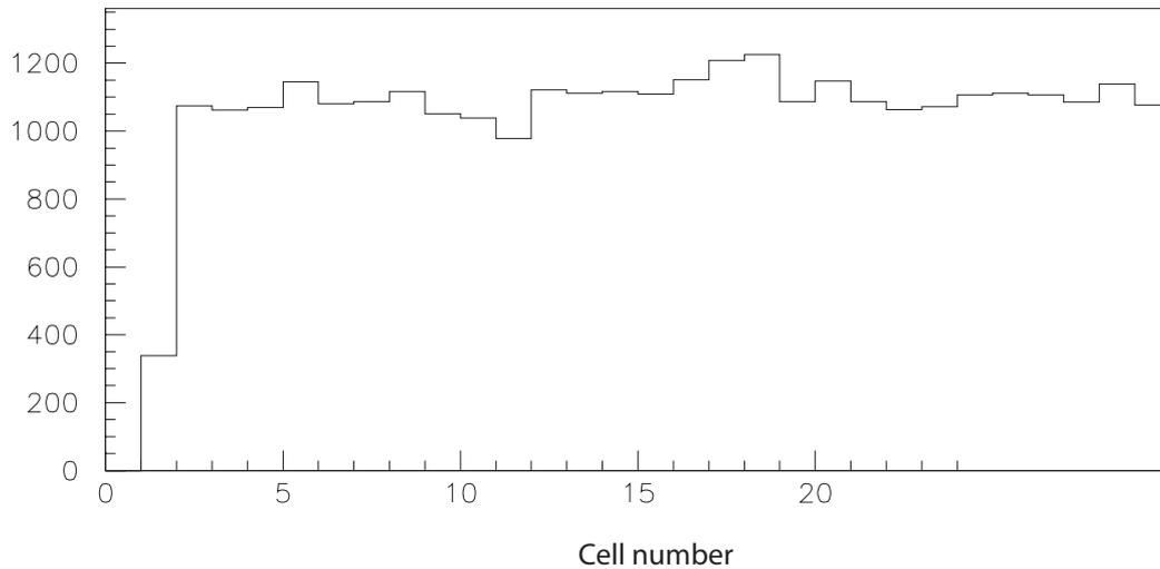
**Figure 3-** Occupancy of the first half of the layer 2 of SL 2 for vertical cosmic. The second half is not shown since HV was disconnected.
