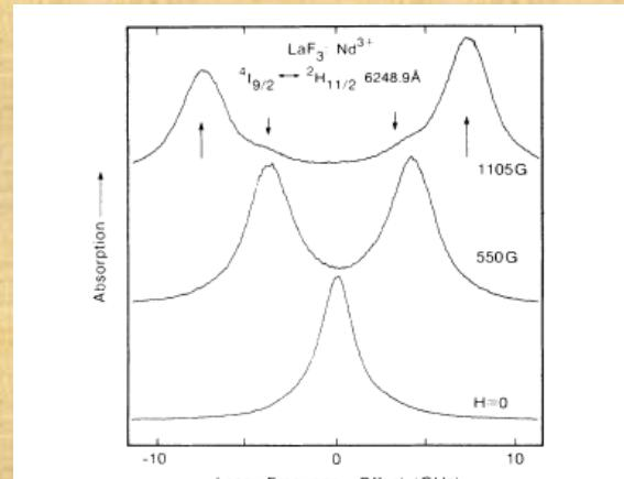
FIG. 3. Zeeman splitting of the 6248.9-Å absorption arising from the transition from the lowest component of  $^4I_{9/2}$  to the lowest component of  $^2H_{11/2}$ .
