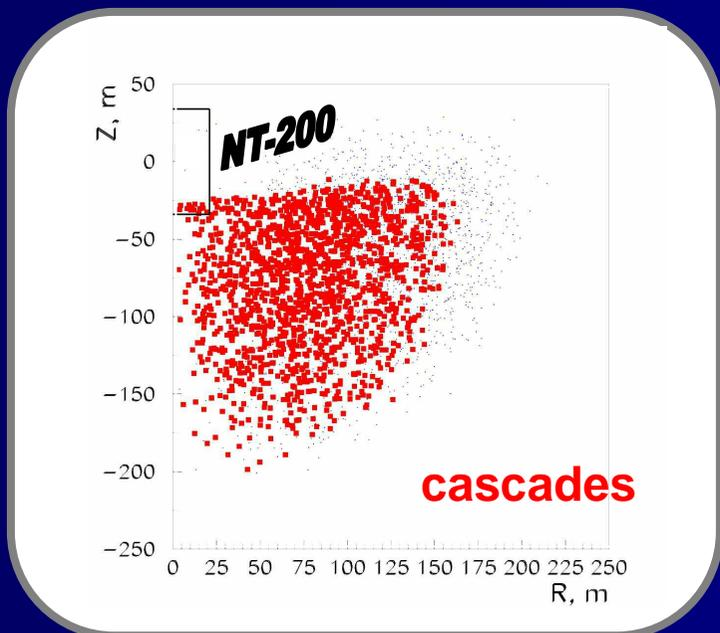
Detection of high energy cascades outside the instrumented volume
