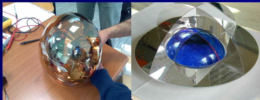
Segmentation of photo cathode of 10" PMT
