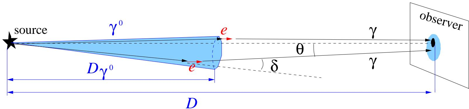
$$D_{\gamma^0} = \frac{1}{n_{IR}\sigma_{PP}} \propto 15 \text{ Mpc} \frac{40 \text{ TeV}}{E} \frac{10 nW / (m^2 sr)}{(vF(v))_{IR}} \quad D_\gamma = \frac{1}{n_{IR}\sigma_{PP}} \propto 400 \text{ Mpc} \frac{1 \text{ TeV}}{E} \frac{10 nW / (m^2 sr)}{(vF(v))_{IR}}$$
