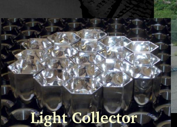
PSF:  $\sim 0.06^\circ$  FWHM measured at Polaris (elevation  $31^\circ$ )
